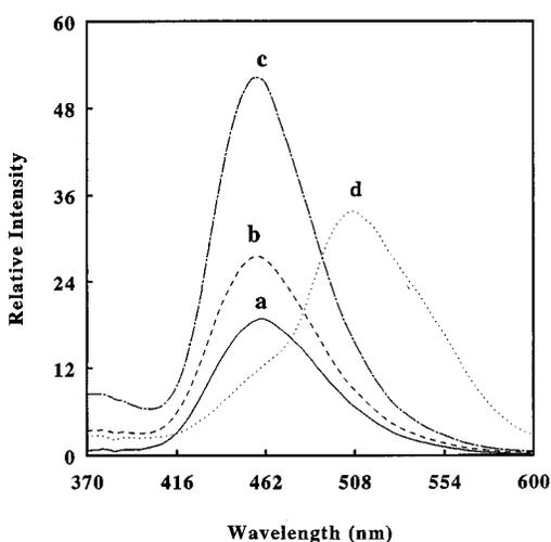
**Figure 6.** Emission of HBT in (a) water (pH 7.0), (b) 8.0 mM  $\beta$ -CD<sub>x</sub>, (c) 8.0 mM  $\beta$ -CD<sub>m</sub>, and (d) 8.0 mM  $\gamma$ -CD<sub>x</sub>.  $\lambda_{\text{exc}} = 340$  nm.
