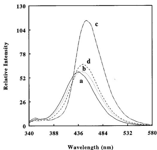
**Figure 5.** Emission of HBI in water (pH 7.0) and in the presence of (b) 8.0 mM  $\beta$ -CD<sub>x</sub>, (c) 8.0 mM  $\beta$ -CD<sub>m</sub>, and (d) 8.0 mM  $\gamma$ -CD<sub>x</sub>.  $\lambda_{\text{exc}} = 330$  nm.
