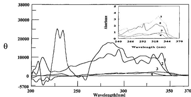
**Figure 3.** Induced circular dichroism (ICD) spectra of  $\beta$ -CD<sub>m</sub> (9.0 mM) with (1) MBT, (2) HBO, (3) HBT, and (4) HBI. (inset) Corresponding absorbance spectra of the molecules in 9.0 mM  $\beta$ -CD<sub>m</sub>, from 240 to 370 nm.
